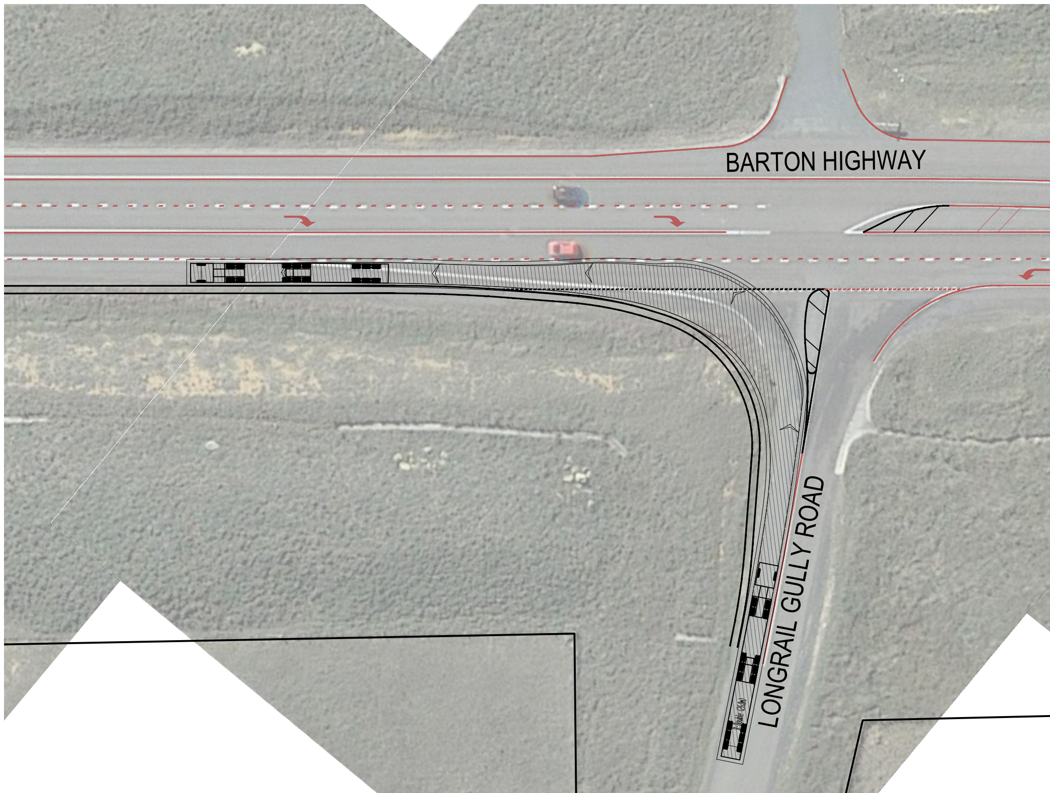
26m B-DOUBLE VEHICLE TURNING PATH - LONGRAIL GULLY ROAD TO BARTON HIGHWAY NORTHBOUND
